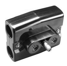
**Model 7013 quick disconnect plug.** QPL LISTED PER MS3349-2 AND MIL-P-18148. The Rebling 7013 quick disconnect plug is a two-wire plug connector for use with lead-acid and nickel-cadmium aviation batteries. They are designed to mate with Rebling Type 7002 series aero battery receptacles and all other receptacles meeting specification MS3509.
